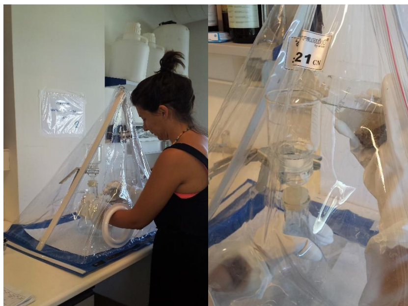
Figure 14: Separation of SMP in the laboratory in Greece, where chamber were used to protect the sample before air born microplastic contamination. Photo: HCMR.
