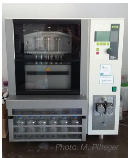
Figure 16: Pressurized Fluid Extractor (acquired from the DeFishGear project). Photo: UNG.
