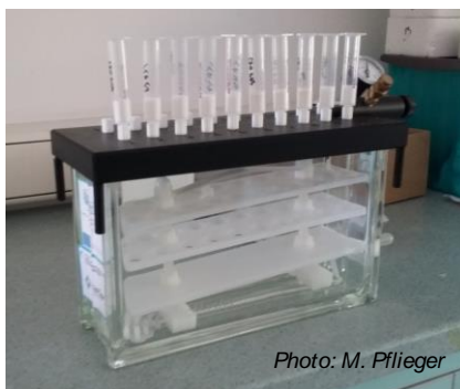
Figure 17: Solid-Phase Extractor (acquired from the DeFishGear project). Photo: UNG.
